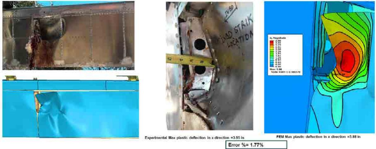
Fig. 15 | Correlation of deformation experiment with simulation
