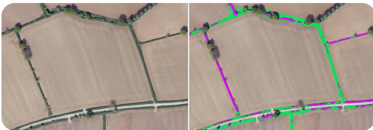
Figure 3: Classified results for the buffer model trained over APGB 25cm imagery showing grass verge and hedgerow predictions.
